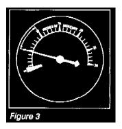
A vacuum reading at idle much lower than normal can indicate leakage through intake manifold gaskets, manifold-to-carburetor gaskets, vacuum brakes or the vacuum modulator. Low readings could also be very late valve timing or worn piston rings. See figure 3.
