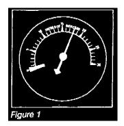
At idling speed, an engine at sea level should show a steady vacuum reading between 14" and 22" HG. A quick opening and closing of the throttle should cause vacuum to drop below 5" then rebound to 23" or more. See figure 1.
