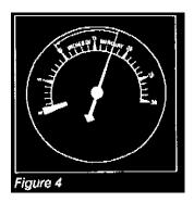
With the engine Idling, the vacuum gauge pointer will drop sharply, every time the leak occurs. The drop will be from the steady reading shown by the pointer to a reading of 10" to 12" Hg or less. If the leak Is between two cylinders, the drop will be much greater. You can determine the location of the leak by compression tests. See figure 4.
