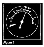
With the engine idling, continued fluctuation of 1 to 2 inches may indicate an ignition problem. Check the spark plugs, spark plug gap, primary ignition circuit, high tension cables, distributor cap or ignition coil. Fluctuations of 3 to 4 inches may be sticking valves. See figure 2.
