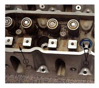
The crack location can be found in any of the five cylinder head(s) oil drains. This can be seen as a clean or shiny area, on an otherwise stained surface (1). Pressurizing the cooling system at this time may reveal coolant, air, or a combination, weeping in the described area. If inspection reveals evidence of coolant witness marks (1), replace the entire cylinder head(s) assembly.
