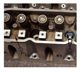
If the cylinder head(s) is a Castech casting (1), inspect the area around the five oil drain holes for witness marks indicating coolant seepage over time
