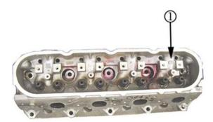
Refer to the illustrations on how to identify Castech casting and/or the very specific areas of the cylinder head(s) for a coolant leak from porosity.
